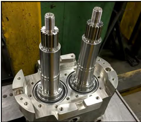
Figure 192 - Shafts seated in gearcase
