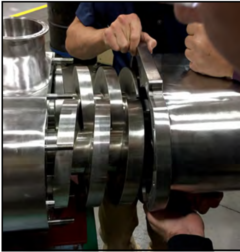
Figure 129 - 220-UTS Install pump cover
