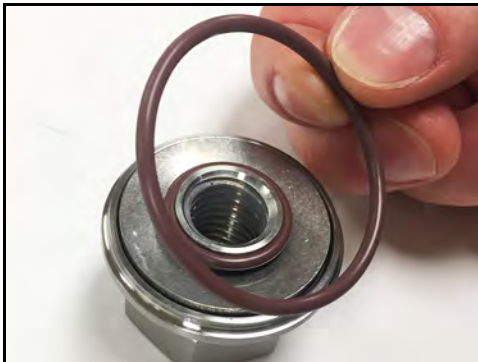
Figure 116 - Install screw nut O-ring
