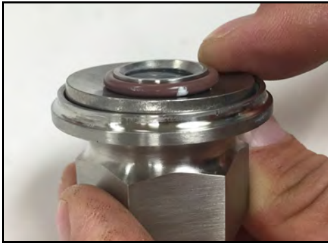
Figure 115 - Belleville washer installed
