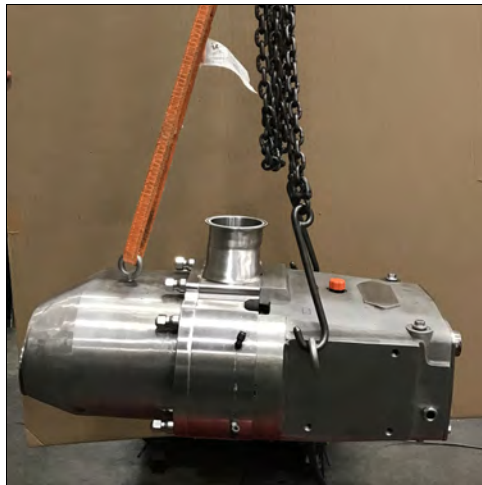
Figure 3 - Lifting location - 130, 220-UTS
