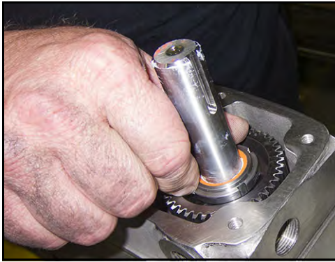
Figure 205 - Install locking nut
