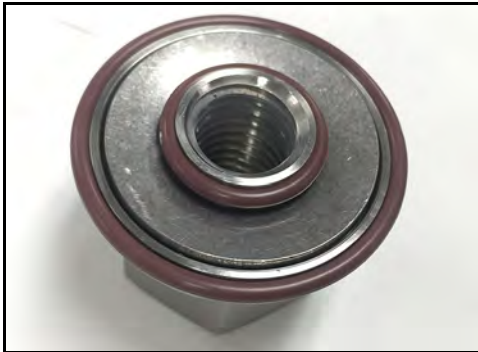
Figure 117 - Screw nut assembly
