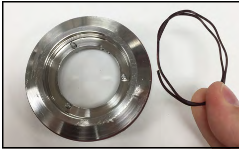
Figure 60 - Seal wave spring
