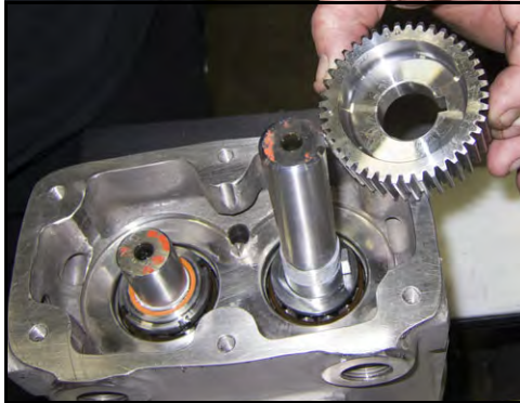
Figure 202 - Install drive gear
