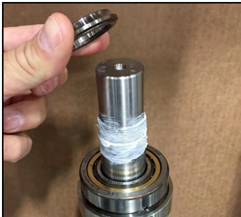
Figure 168 - Place race on shaft
