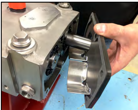
Figure 235 - Install gear case cover
