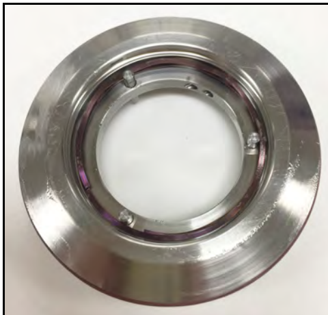
Figure 67 - Seal wave spring installed
