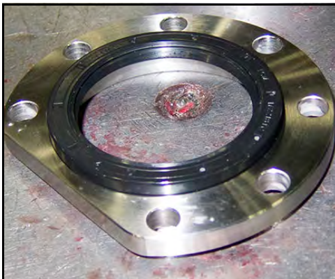
Figure 193 - Center bearing retainer seal
