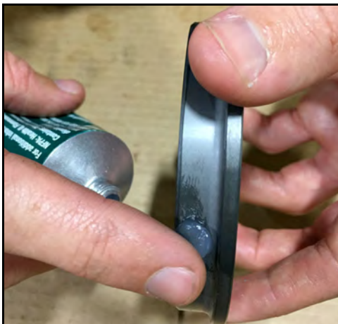
Figure 81 - Lubricate the outer diameter of the seal
