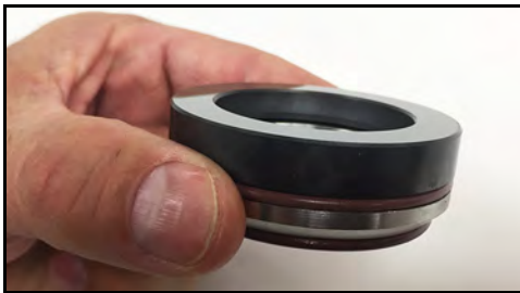
Figure 102 - Seal seat installed on seal cap
