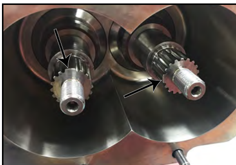
Figure 108 - Align screw and shaft spline
