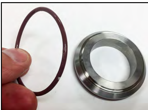
Figure 45 - Remove cap-to-screw O-ring
