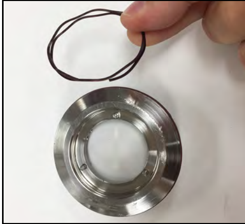
Figure 66 - Seal wave spring
