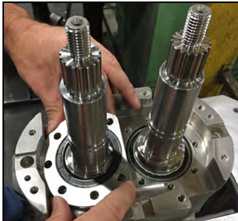
Figure 199 - Install bearing retainer
