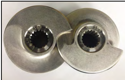
Figure 107 - Arrange screws: LH-RH
