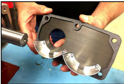
Figure 234 - Place gasket on cover
