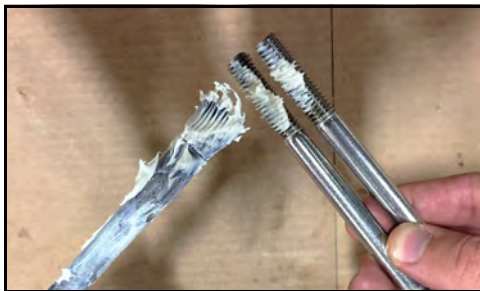
Figure 89 - Apply anti-seize to threads
