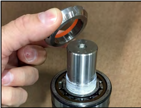
Figure 178 - Place locking nut onto shaft
