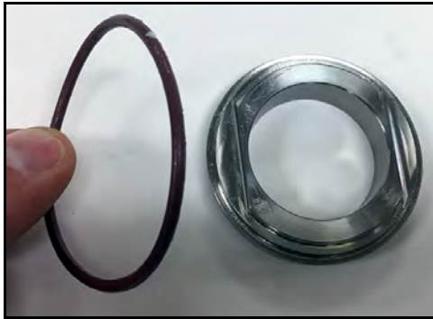
Figure 46 - Remove cap-to-seat O-ring
