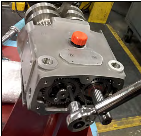
Figure 227 - Torque locking assembly bolts
