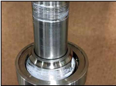
Figure 164 - Race pressed on shaft
