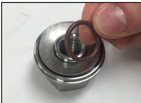
Figure 114 - Install washer retainer O-ring
