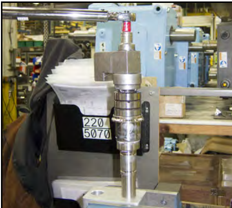
Figure 179 - Torque down locking nut
