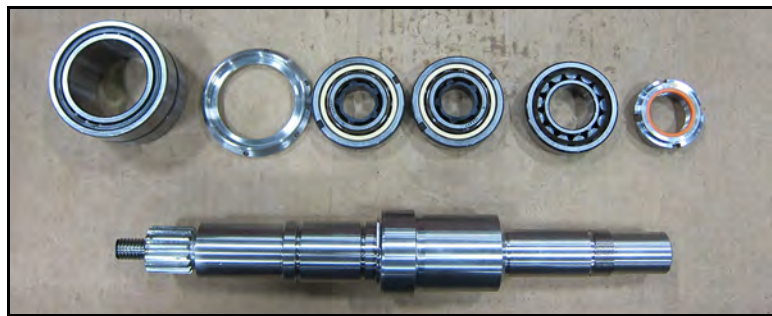
Figure 151 - Short Shaft: Assembly items needed
