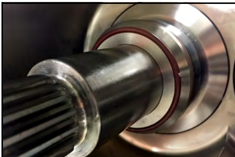
Figure 104 - Seal cap installed on shaft
