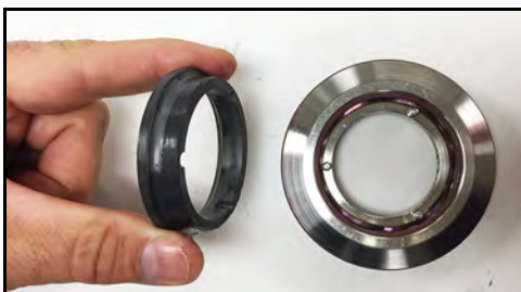
Figure 73 - Lubricate and install seal
