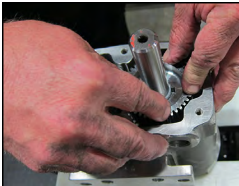
Figure 203 - Install drive gear
