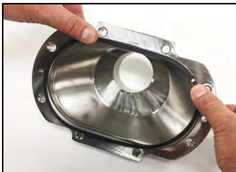
Figure 127 - Install cover gasket
