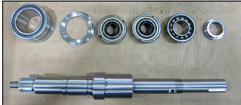
Figure 150 - Drive Shaft: Assembly items needed
