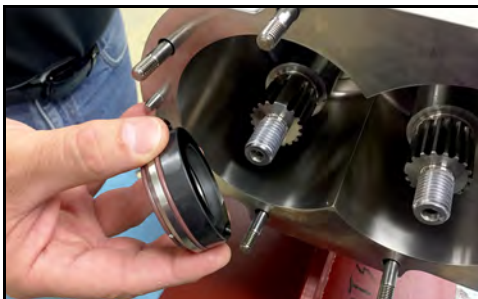
Figure 103 - Install seal cap assembly
