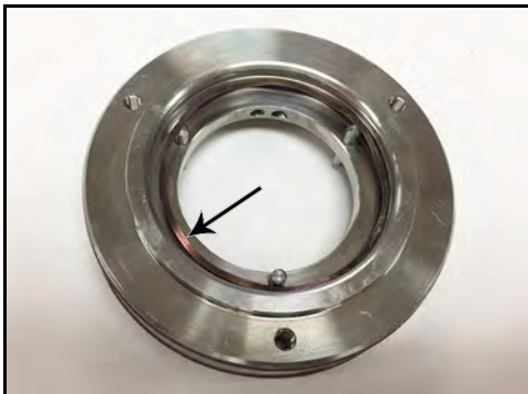
Figure 71 - Seal wave spring installed
