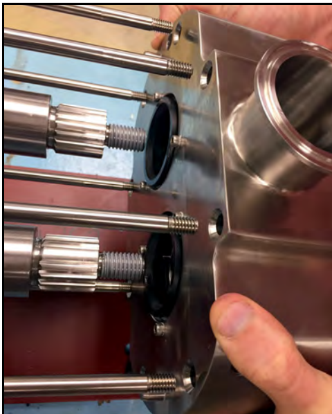
Figure 87 - Install pump body onto shafts
