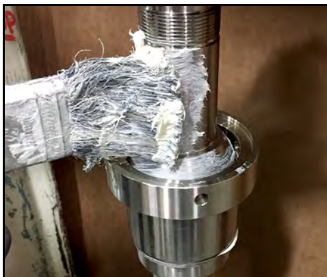
Figure 161 - Apply anti-seize to shaft
