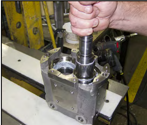
Figure 186 - Place short shaft in bore
