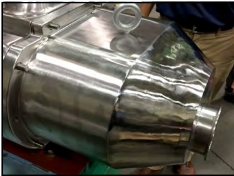
Figure 130 - Seat pump cover against pump body
