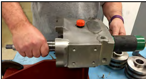
Figure 147 - Tap short shaft out of gear case
