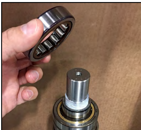
Figure 177 - Place bearing onto race
