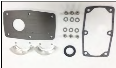
Figure 229 - Gear case cover components
