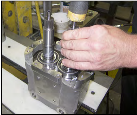
Figure 191 - Tap shafts to center in bores
