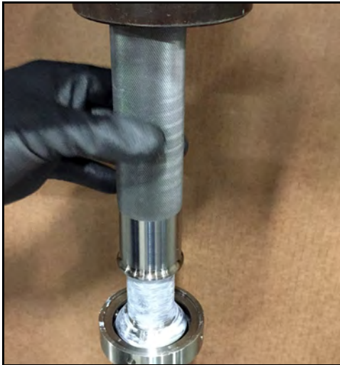
Figure 163 - Press race onto shaft
