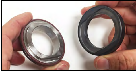
Figure 101 - Line up seal cap and seal seat
