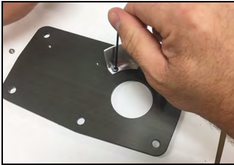
Figure 232 - Tighten shroud screws
