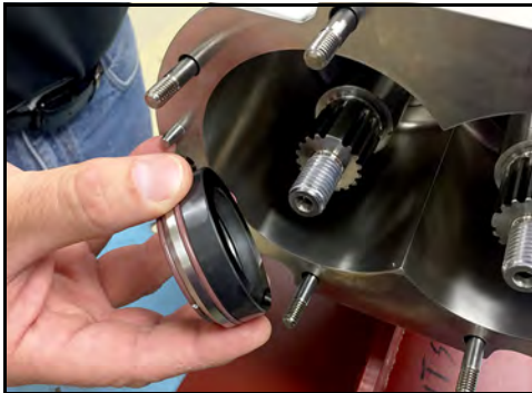
Figure 43 - Remove seal cap assembly
