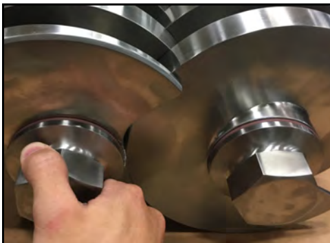
Figure 124 - Install screw nuts
