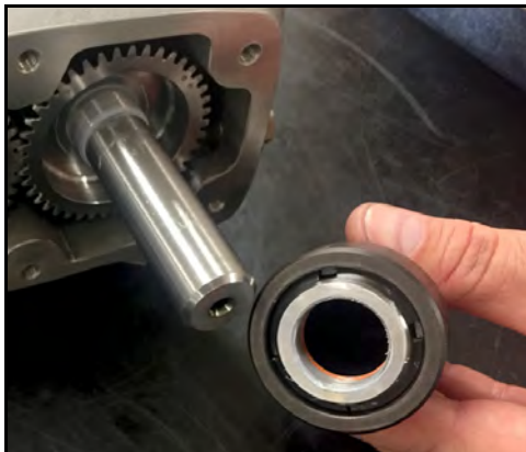
Figure 142 - Remove locking nut and gear
