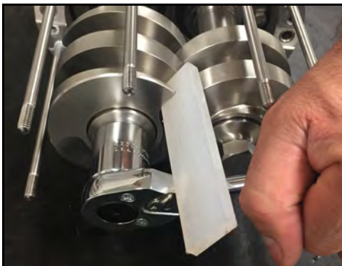
Figure 219 - Tighten screw nut
