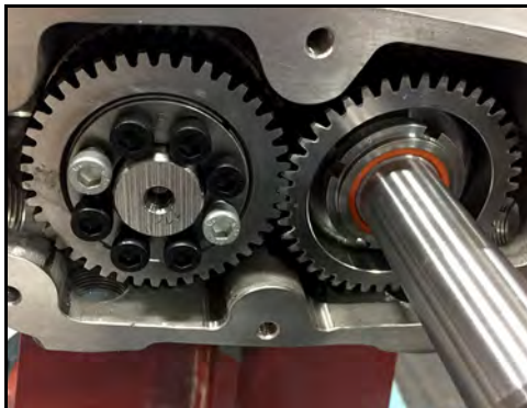
Figure 214 - Align loose gear with drive gear
