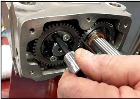
Figure 137 - Loosen bolts in locking assembly
