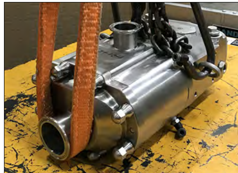
Figure 2 - Lifting location detail - 015, 030-UTS
