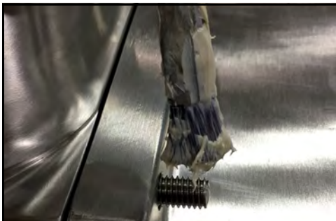
Figure 131 - Apply anti-seize to threads
