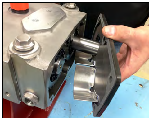
Figure 135 - Remove gear case cover
