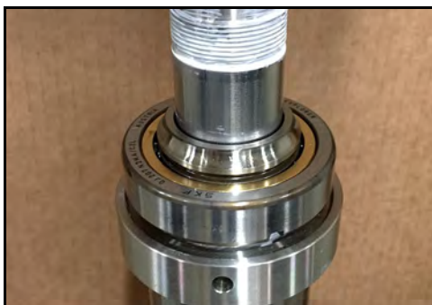
Figure 169 - Press race into bearing
