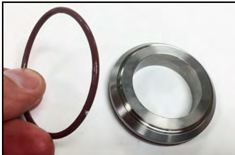
Figure 99 - Install cap-to-screw O-ring
