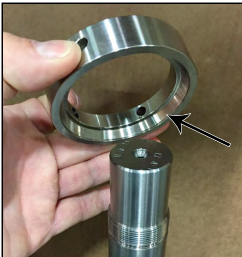
Figure 157 - Place bearing spacer on shaft
