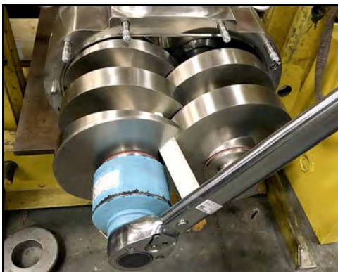
Figure 125 - Torque left screw nut
