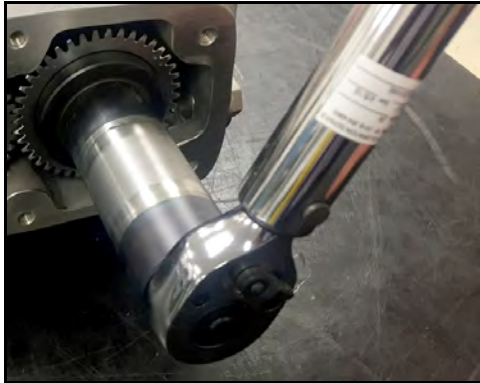
Figure 141 - Loosen locking nut
