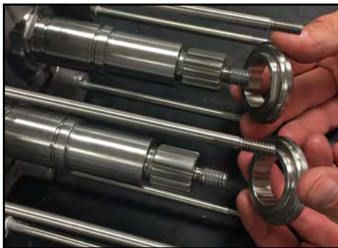
Figure 215 - Install seal caps
