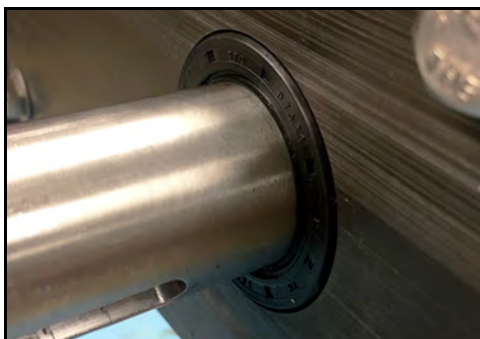
Figure 239 - Oil seal installed
