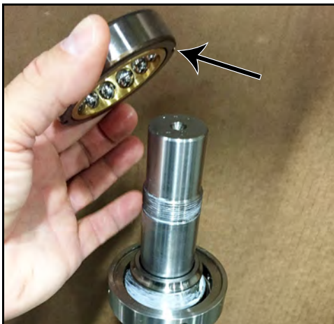
Figure 165 - Place bearing onto race
