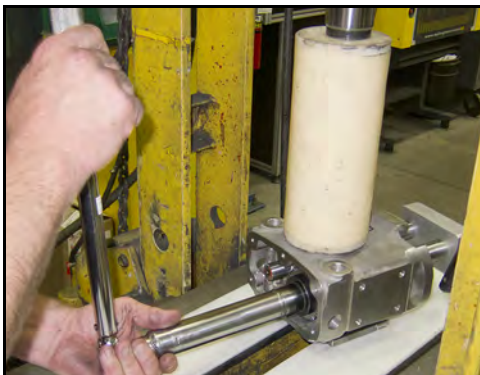
Figure 207 - Torque locking nut
