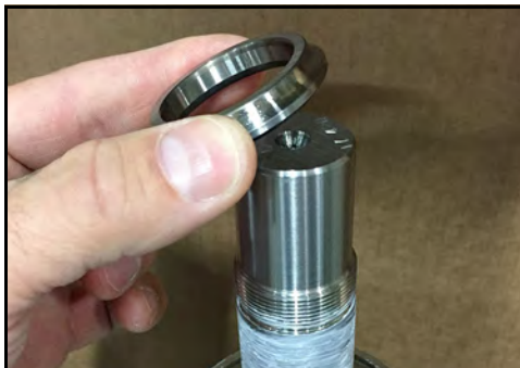
Figure 162 - Place race onto shaft
